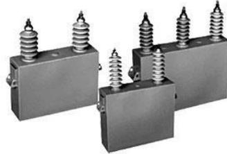
**Composition:** A capacitor is a passive two-terminal electrical component used to store energy in an electric field. The forms of capacitors vary widely, but all contain at least two electrical conductors separated by a dielectric (insulator). Most large capacitors consist of metal foils separated by a thin layer of insulating film. Prior to 1979, capacitors contained PCB oil as a dielectric fluid.
